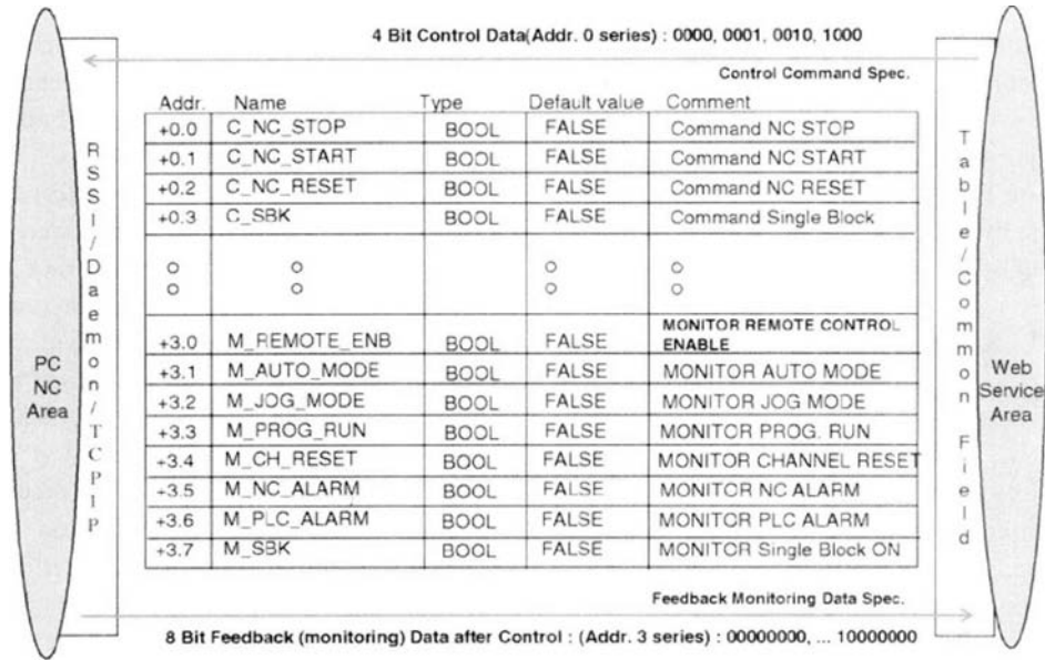
Fig. 11 Interface protocol for remote control
